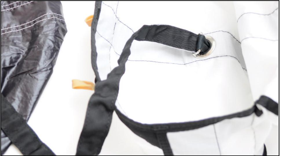
Install the malleon to the inside of the D-bag as shown, around the bridle and through both loops.
